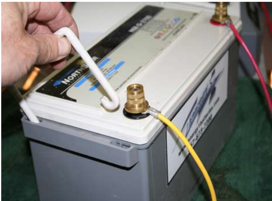
The Energy 1's carrying handles detach from the case too easily.
